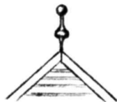
FINIAL AT ROOF RIDGE
