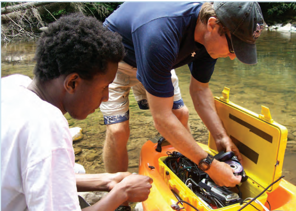
Top: Dr. Paul Ayers mapping habitat on Abrams Creek (GRSM) using kayak equipped with underwater video camera and GPS unit in storage compartment. Photo credit: Ray Albright Bottom: Dr. Paul Ayers and University of Tennessee student, Samba Nyika, check video and GPS equipment in kayak. Photo credit: Ray Albright
