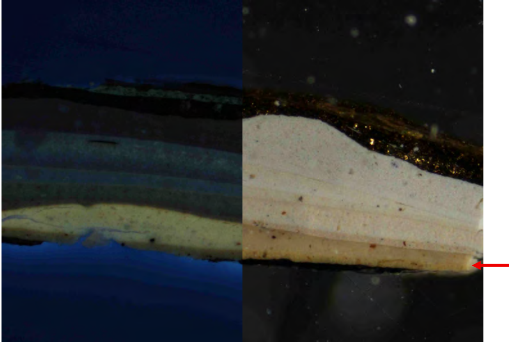
Figure 18. The metal grille in the elevator was originally painted with grayish orangish yellow (arrow). It was only painted gold in the most recent paint scheme. BB.E2 (elevator), ultraviolet light (L), visible light (R), 40x magnification.
