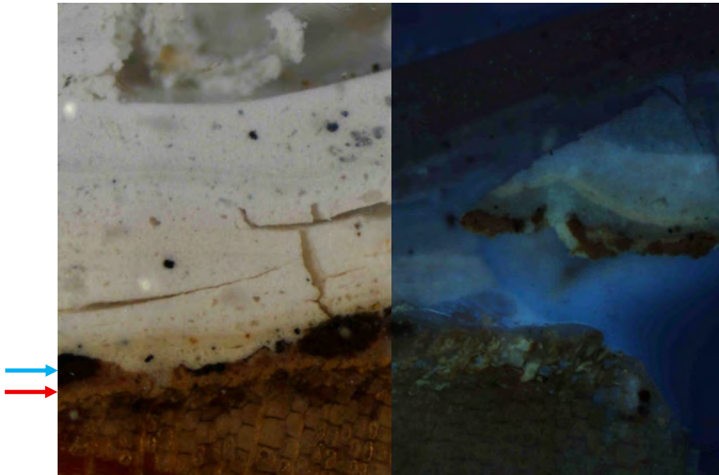
Figure 11. The sample from the fanlight sash suggests that the original finish is a brownish orange paint/stain (red arrow) topped with a transparent coating (blue arrow), creating an overall appearance of glossy very dark purplish brown. BB.EXT. 22, visible light (L), ultraviolet light (R), 40x magnification.
