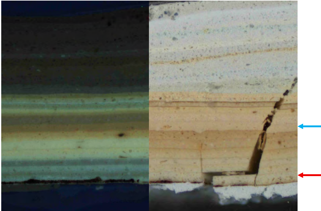
Figure 32. A representative sample of the metalwork originally painted brownish white (arrow), removed from the paneled capital center. The blue arrow indicates the light orange yellow that likely matches the earliest existing layer on the partition cornice. BB.106.3 (Men's Bath Hall), ultraviolet light (L), visible light (R), 40x magnification.
