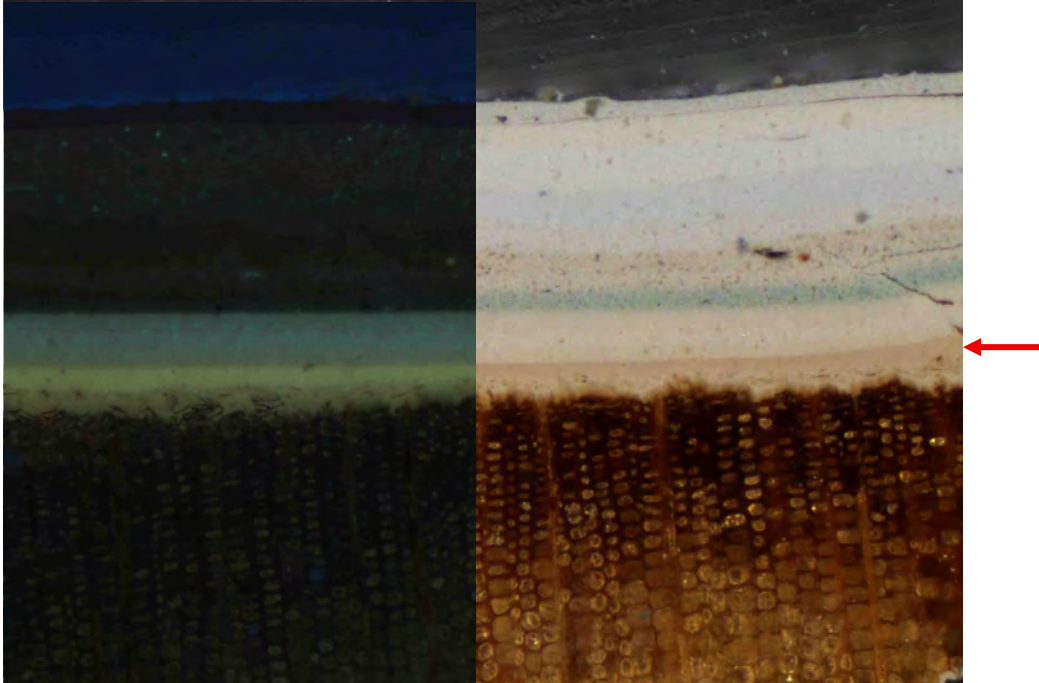
Figure 42. The partition sample contains two fewer layers than the plaster wall sample, suggesting that the partition was installed early. The earliest existing finish on the partition is a moderate orange yellow (arrow) that appears to match the third layer on the plaster (see Figure 41). BB.200.13 (2F Lobby), ultraviolet light (L), visible light (R), 40x magnification.
