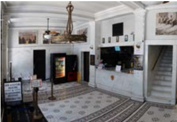
Figure 1.C.2. Character-defining features of the interior that can be seen in the lobby (100) include flat plaster walls and ceilings, decorative plasterwork (pilaster capitals, paneled beam casings), mosaic tile floors, marble wainscoting and wall panels, marble staircases with brass hardware, and the original elevator (cab, doors, and hardware).
