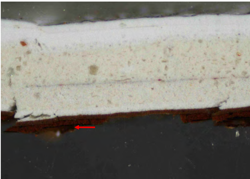
Figure 39. The metal windows were finished in a dual white and brown color scheme like the wood windows. The metal window transom, pictured, was originally painted in dark grayish reddish brown (arrow), likely intended to match the naturally finished wood window sash. BB.109.8 (Men's Cooling Room), visible light, 40x magnification.
