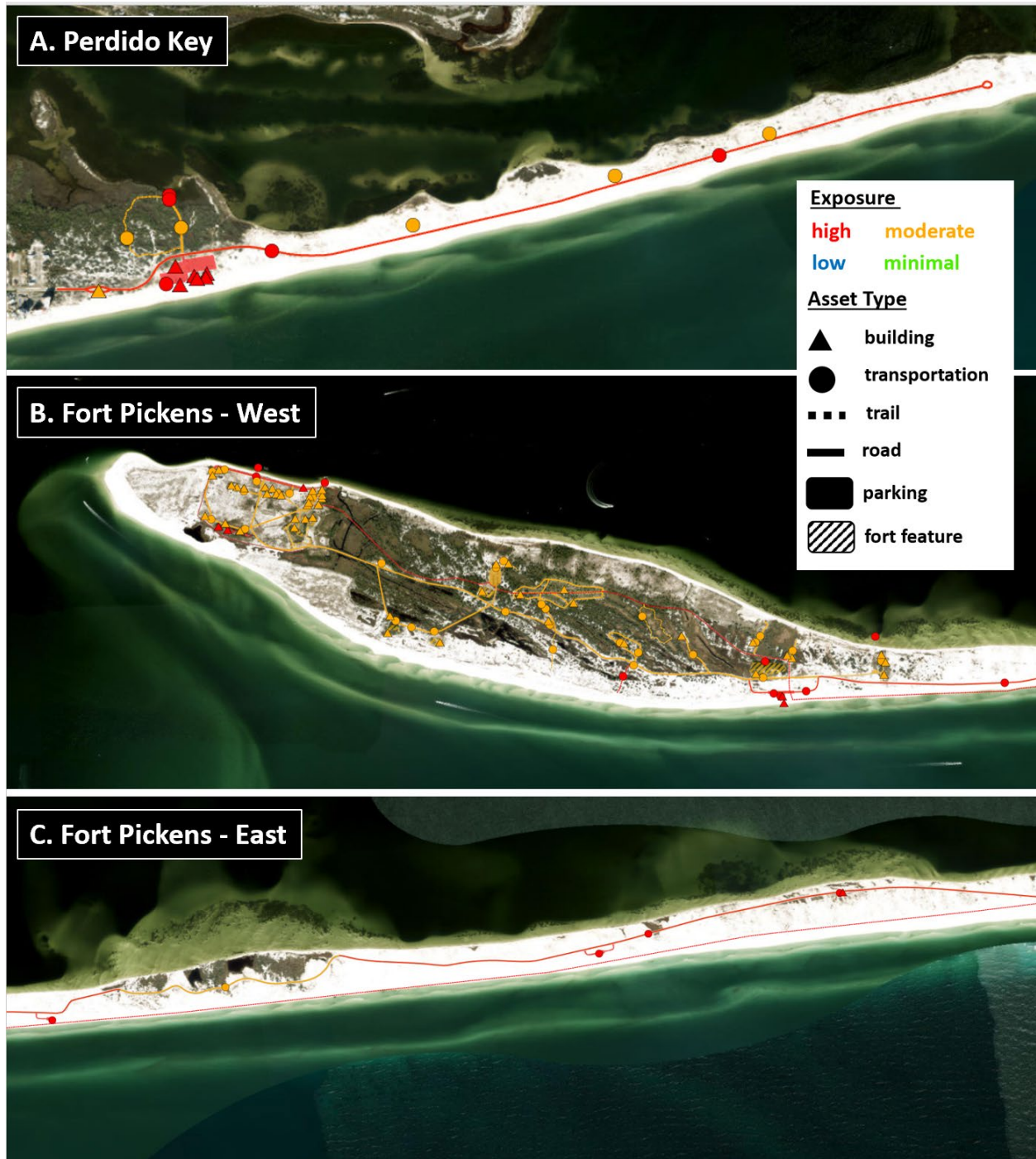
Figure 2. GIS exposure results summary for the A) Perdido Key (Fort McRee area not shown), B) Fort Pickens - West, and C) Fort Pickens - East areas of the FL district. Background is 2021 ESRI world imagery.
