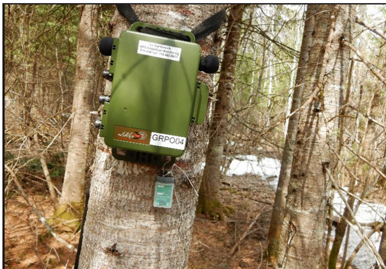
An automated recorder, or “frog logger.” Microphones come out of the top left and right of the box. A temperature logger is attached below. NPS PHOTO
