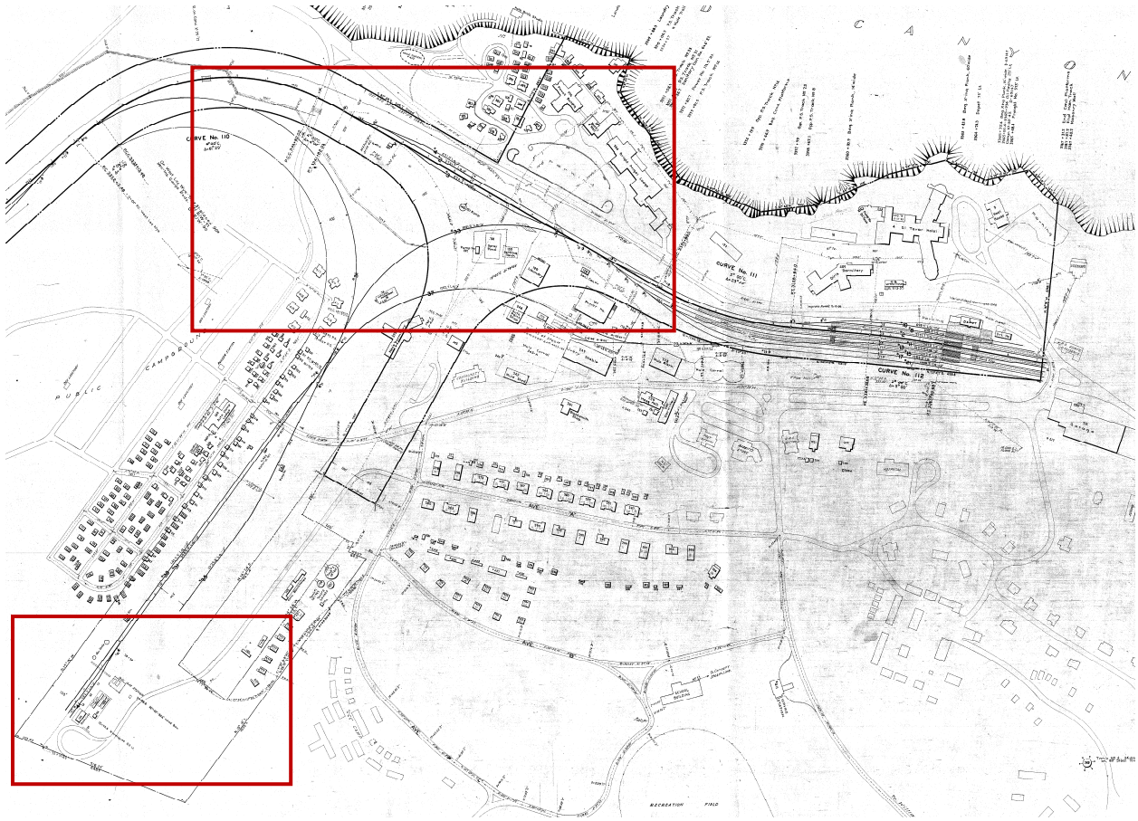
Figure 10. Map of realigned wye overlaid by the trace of the old wye. See next page for enlarged views of the outlined areas. Detail from "Grand Canyon Station Plat," ATSF Drawing No. CECL 1-21497, Jan. 10, 1938, Grand Canyon National Park Museum Collection, GRCA 107608.
