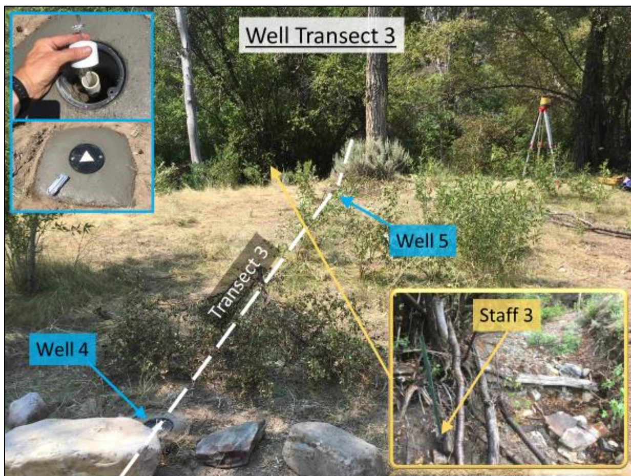
Figure 10.1. Groundwater well Transect 3 as an example. Wells 4 and 5 (top-left inset) were installed in the floodplain at foreground, and Staff 3 (bottom-right inset) was affixed to a t-post in the channel.
