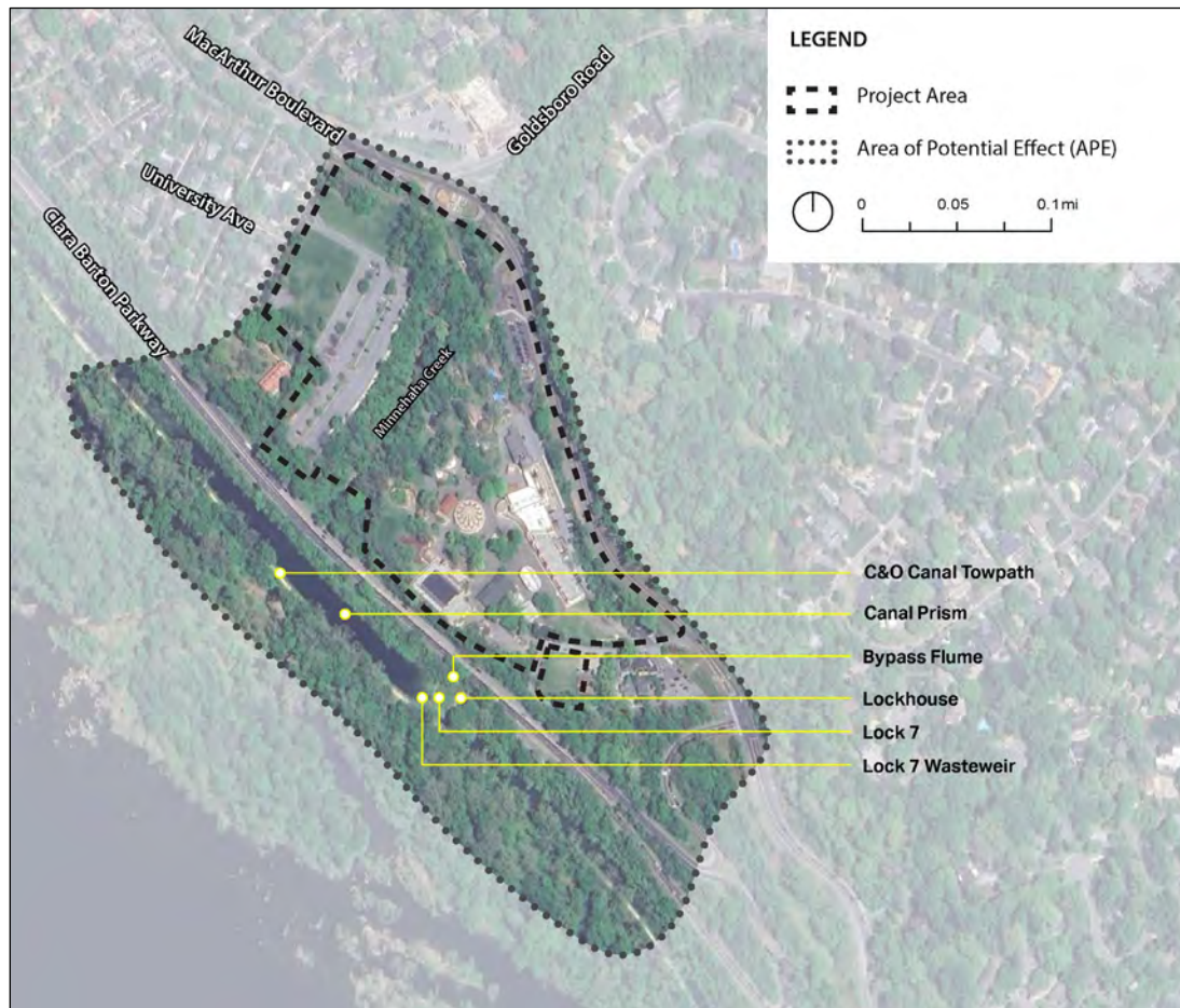
Figure 14: Chesapeake and Ohio Canal National Historical Park Historic District Contributing Elements within the APE
