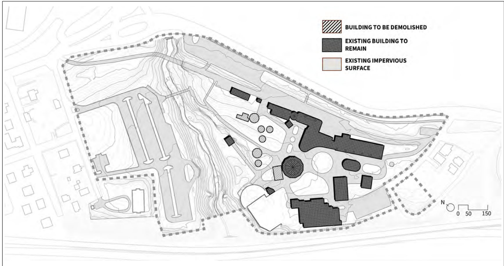
Figure 7: Alternative B – Proposed Building and Structure Removal
