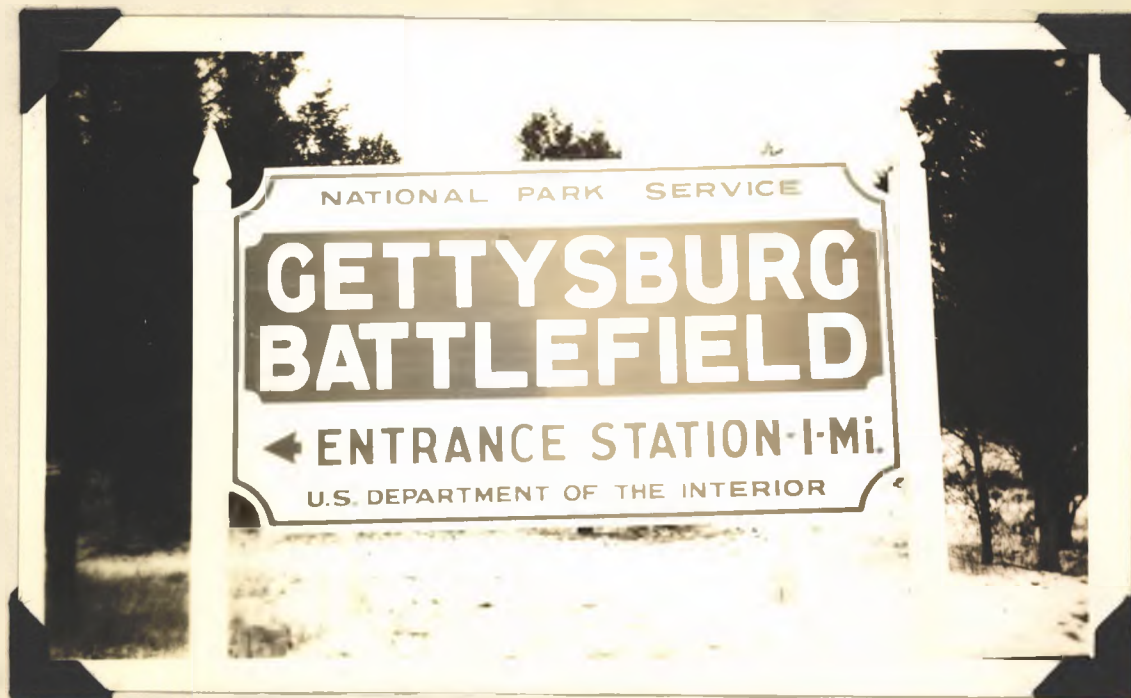
View of New Approach Sign, 5'6" by 10'6", on EMMITSBURG ROAD. Large Lettering, 12".
