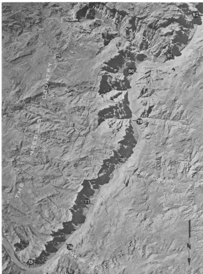
TEXT-FIGURE 66.—Vertical aerial photograph of the Colorado River covering the region from approximately Mile 75 to Mile 81 in Cataract Canyon. The frequent rapids in this section are produced predominantly by slumps of canyon wall instead of debris fans at the mouths of the small canyon.
