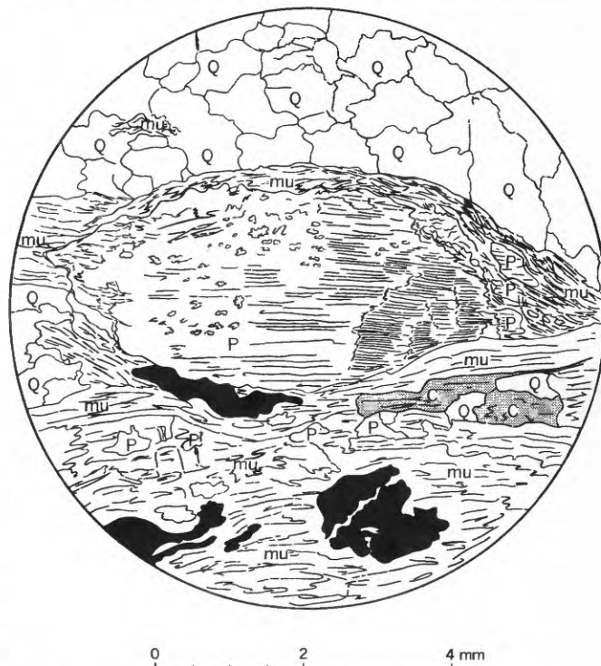
FIGURE 10.—Micrograph of plagioclase porphyroclast in gneiss from north of the Potomac River opposite Hermit Island. P, plagioclase; mu, muscovite; C, chlorite; Q, quartz.
