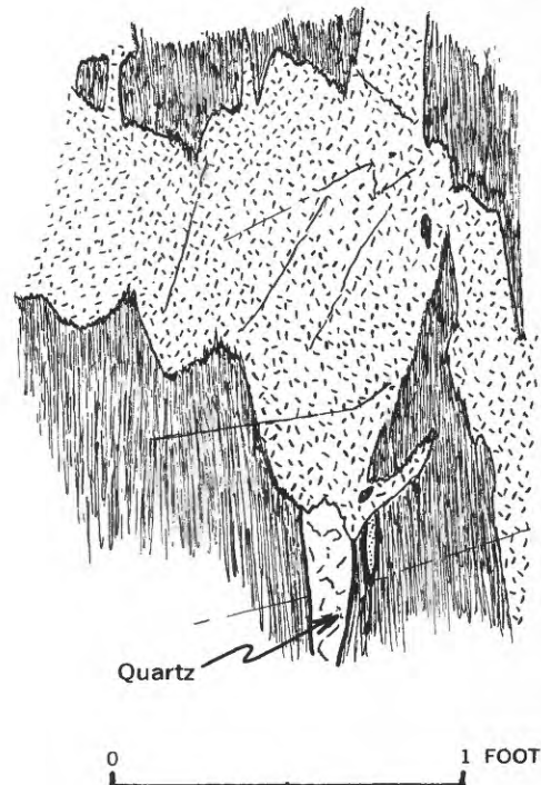
FIGURE 12.—Sketch of irregular dike of even-grained granodiorite in schist near the northeastern end of Bear Island. The granitic rock is unfoliated and its contacts with the schist are indefinite in detail. Septa of schist extend into and nearly across the dike.
