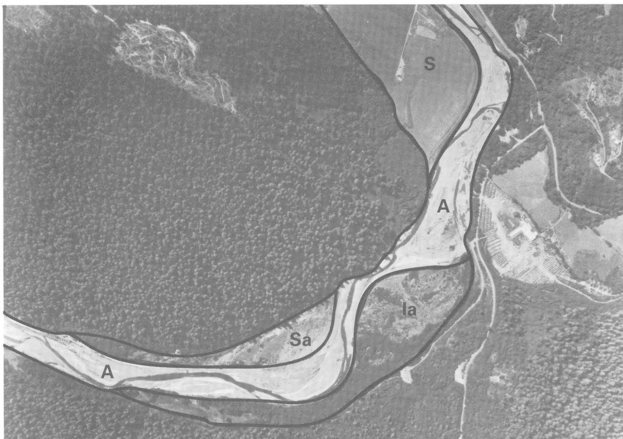
FIGURE 6.—Classification of sediment reservoirs shown on a vertical aerial photograph (1978; scale 1:6,000) of Redwood Creek, kilometer 100 near Orick; flow is from left to right. Classes are active (A), semiactive (Sa), inactive (Ia), and stable (S).
