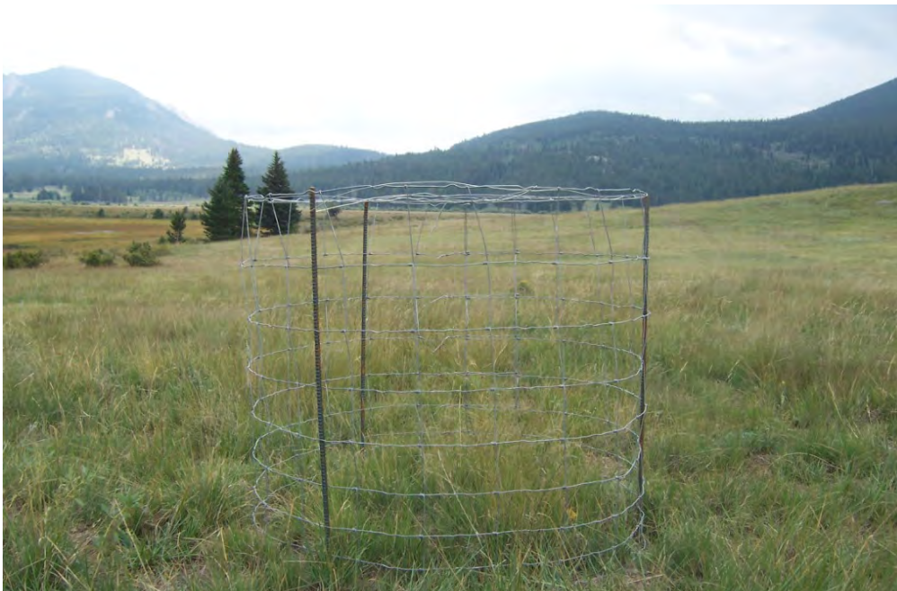
Figure 6.1. Photo of grazing cage design currently being used in elk-vegetation monitoring program.
