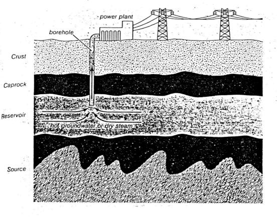
Schematic view of a dry (steam) or wet (hot water or brine plus steam) geothermal well and power plant.
