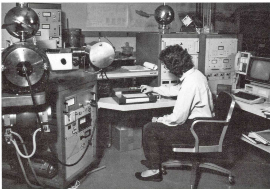
A technician of the U.S. Geological Survey uses a mass spectrometer to determine the proportions of neodymium isotopes contained in a sample of igneous rock.
