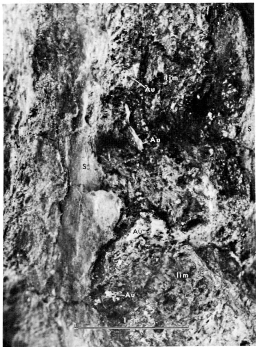
B. Wire gold (Au) in limonite (lim) pseudomorphs after disseminated pyrite, in altered sericite schist (s). USNM 80171, labeled "Potomac Mine." Possibly from workings along the Potomac vein (pl. 2) or from the Montgomery mine (fig. 1), which was once known as the Potomac mine. Photographs by David Massey, U.S. Geological Survey.
