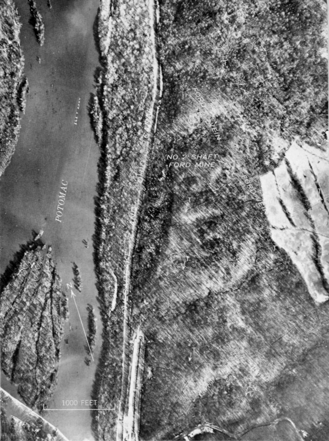
FIGURE 2.—Aerial photograph showing surface workings along part of Great Falls vein system. For location of area, see plate 2. Note pits and trenches along Ford vein and vein to west. Lines of trees in open field east of Ford vein mark outcrops of other quartz veins. Long east-west prospect trenches (T) date from exploration work during 1915-18.
