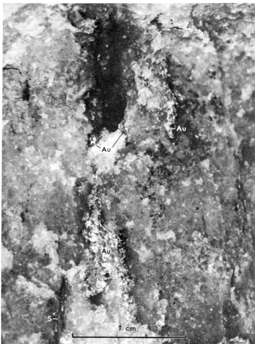
A. Gold (Au) in sheeted vein quartz with schist partings (S). Gold grains are apparently elongated parallel to strong lineation in schist. U.S. National Museum specimen (USNM) 66014 labeled "Montgomery Co., Maryland, gift of George Huddleston, 1880." Possibly from Huddleston mine (fig. 1).
