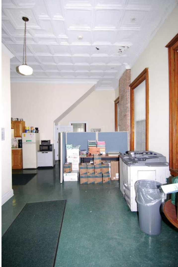
Photo 87. View of historic kitchen space, now administrative area, looking west. Circulation from the central area of the Mess Hall to the Admin/Support area is unencumbered. Short pile carpets are taped down to maintain a continuous path (JMA, October 2009).
