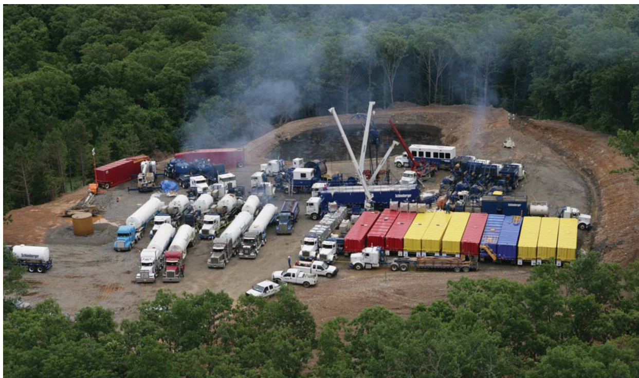
The numerous truck-mounted pumps and temporary storage tanks needed to fracture-treat the Marcellus Shale will require larger well locations. The fracturing equipment and materials on location in this photograph represent over 100 round trips to location by large tractor trailer trucks. (Photo source—Unknown)
