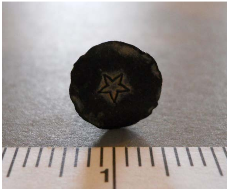
Figure 27. A rivet (NC575) with a star on its base.
