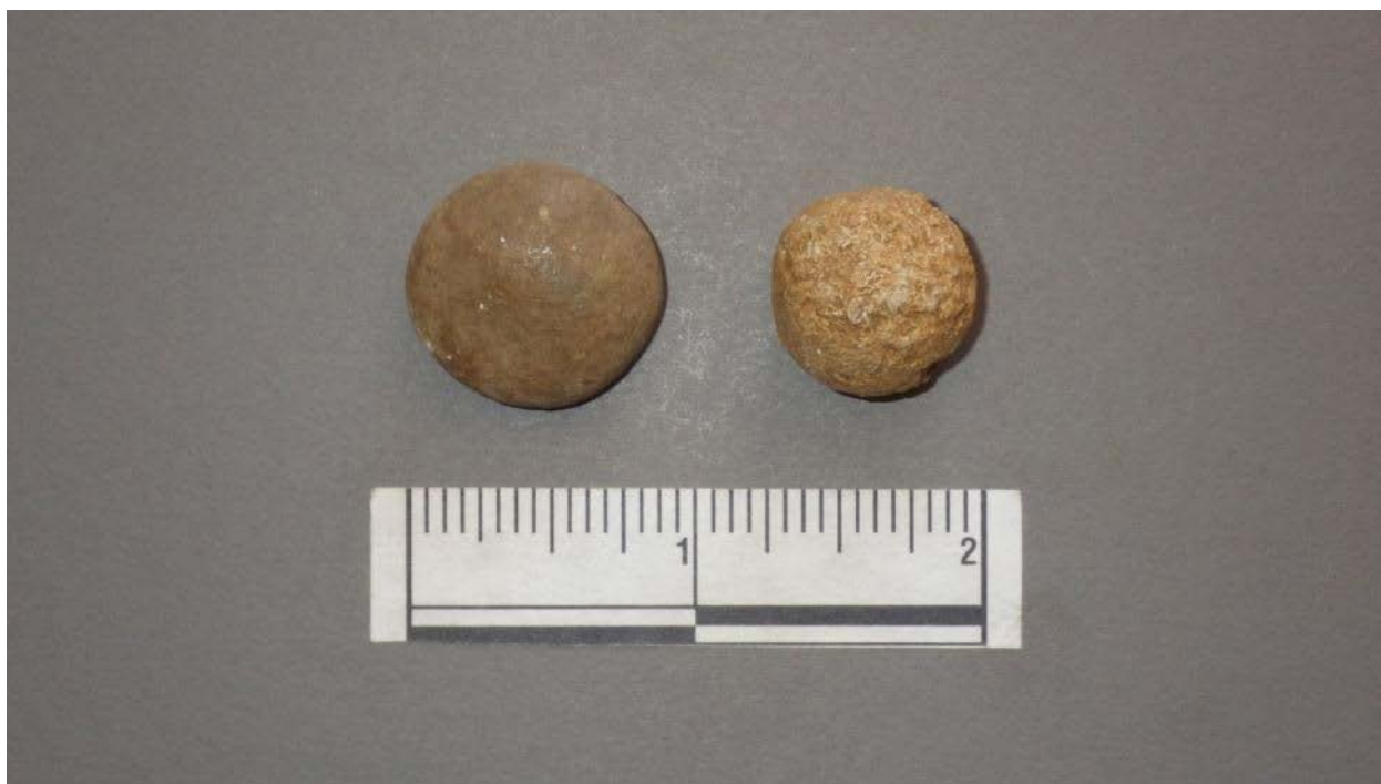
Figure 33. Two shrapnel balls. The ball on the left (NC367) impacted on something solid, while the ball on the right (NC363) impacted a softer object.
