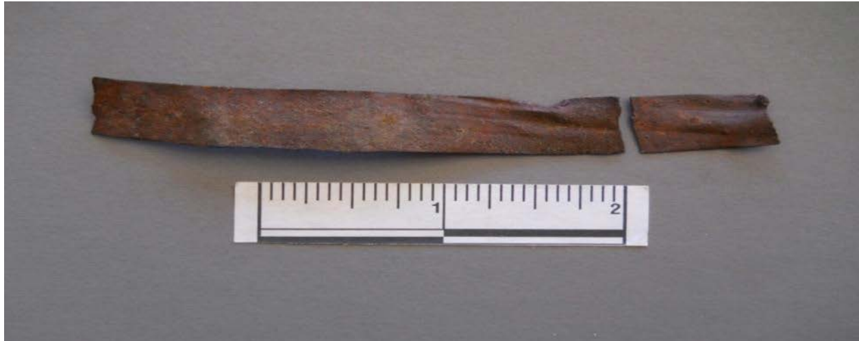
Figure 34. Sabot strap fragment (NC722). Note stretch lines in the metal.
