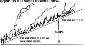
**Terrain**, the shape of the land, has a major affect on fire behavior. *Box canyons*, narrow canyons, and gulches act like a chimney of a stove. Radiation, convection, and spot fires speed up as when a damper was opened in a chimney. This effect can result in *extreme fire behavior* and can be very *dangerous* to firefighters.
