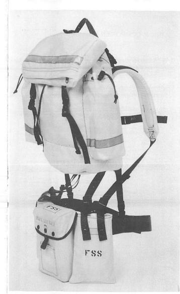
The firefighters field pack is designed for the wild land firefighter. The field pack consists of: (1) pack, (2) harness, (3) equipment belt, (4) two canteen cases, and (5) fire shelter. The field pack allows firefighters to carry all on-line essentials in an efficient, nonrestrictive manner.
