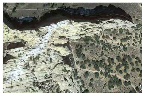
Aerial view of Inscription Rock shows prominent linear joints that provide pathways for water to move through the cliff. Pinon and Juniper trees for scale. Photo courtesy of Google Earth.
