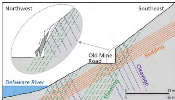
Figure 22. Schematic illustration of rockslide potential along longitudinal joints triggered by removal of the toe of the slope. The road cut along Old Mine Road across from Tocks Island is steeper than the dip of the joints making the areas susceptible to rock falls along the joints. Note that closer to the river the slope is shallower than the dip of the joints, meaning there is little likelihood for rock fall in that area. Graphic by Trista Thornberry-Ehrlich (Colorado State University) redrafted from Epstein (2001a).
