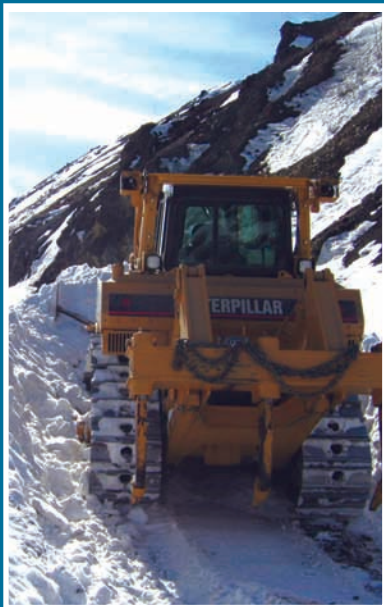
The D7 bulldozer pioneers the first pass up Tattler Grade. It takes more than 11 weeks each spring to clear the 92-mile park road for the operating season.
