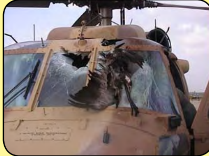
Damage to military helicopter from crane strike.
