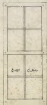
SECOND FLOOR SASH - UPHILL END 2 REQ SCALE 1/4" = 1'-0"
