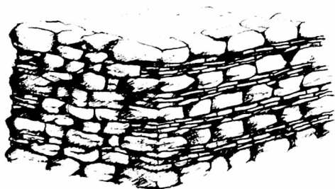
Cored Masonry (Can be seen at Pueblo Bonito and other great houses)
