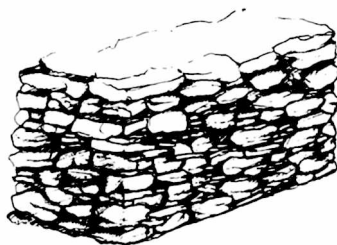
Compound Masonry (Found here and at some great houses)
