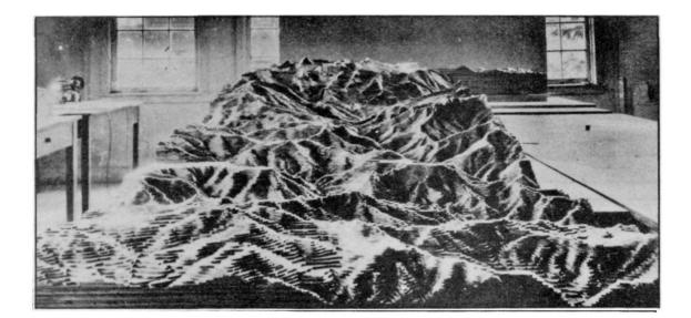
Pattern of Sequoia Relief Model in Process of Construction. The terrain is represented by superimposed cardboard laminations, shaped according to contours (foreground), and then smoothed to simulate the slope of the ground by filling in the steps (background). upon a practical balance between the character of the terrain; the size of the model and the thickness of material available for the laminations.
