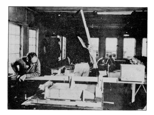
Gluing Down Contour Laminations. This is an improvised press made for the purpose with a  $2 \times 4$  set in supports so that it can be weighted as much as desired. Care should be taken to distribute the pressure over the entire area of the laminations being glued.
