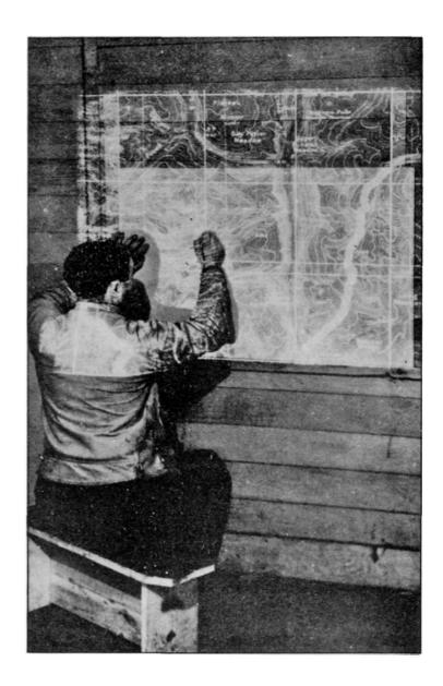
Tracing Contours on a Cardboard Sheet. The original map is transferred to a lantern slide. Then it is enlarged nine times on this cardboard sheet with a projector. cardboard sheet is fastened, and the contours are traced directly onto them. This method is shown on page 13.
