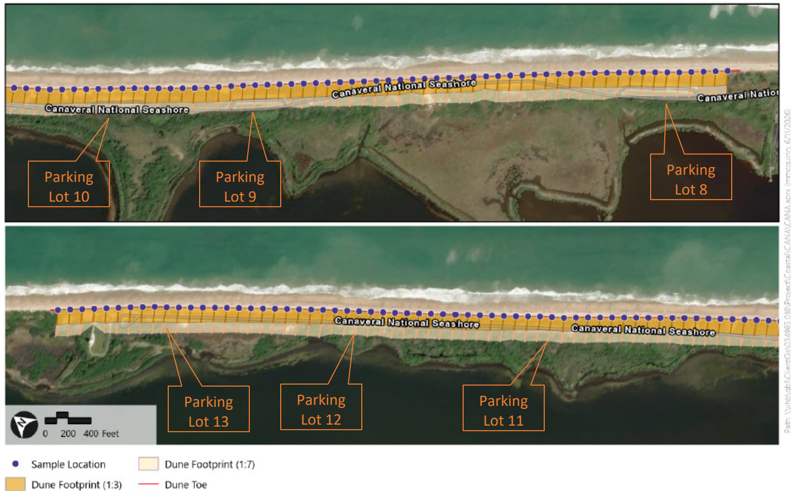
Figure B-1. Approximate dune widths given 1:3 and 1:7 slopes
