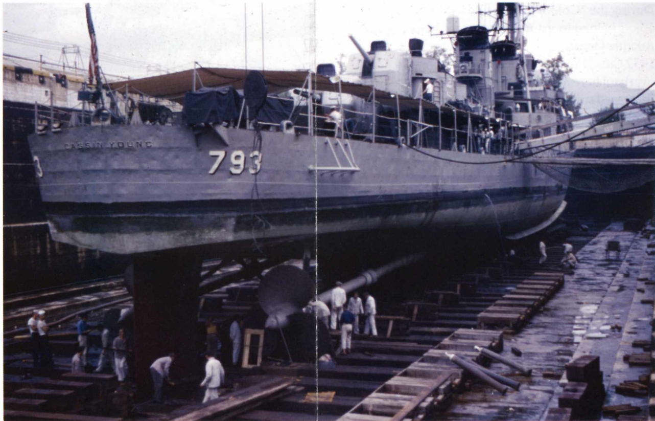
Structural problems with the rudder and propeller required emergency repairs in France in 1959, which eventually lead to her decommissioning a year later.
