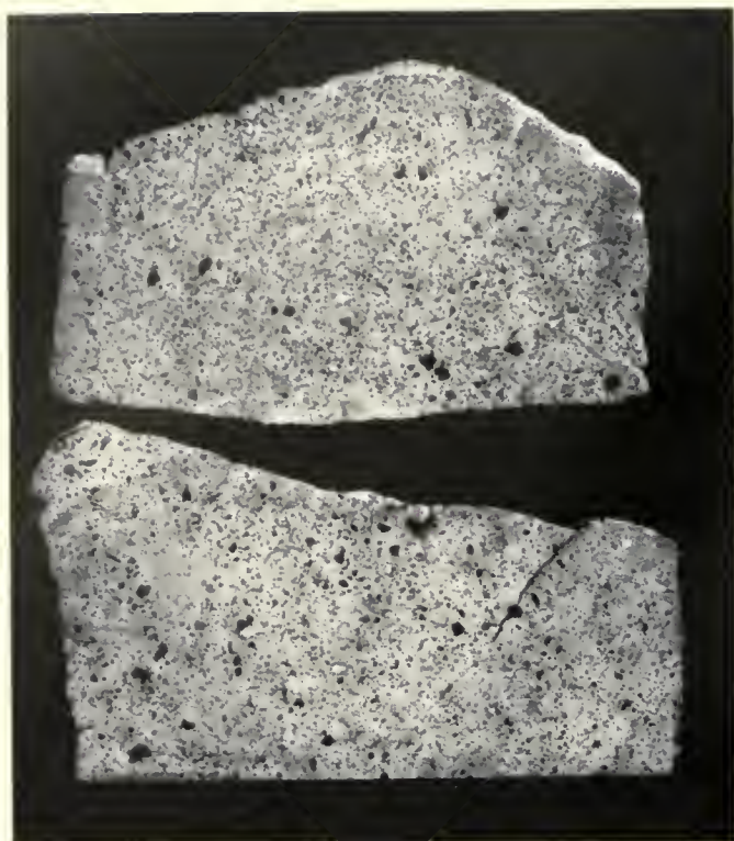
FIG. 31. Photograph of G 4077, a sample of heterogeneous mudstone, showing heterogeneity in both horizontal and vertical sections.
