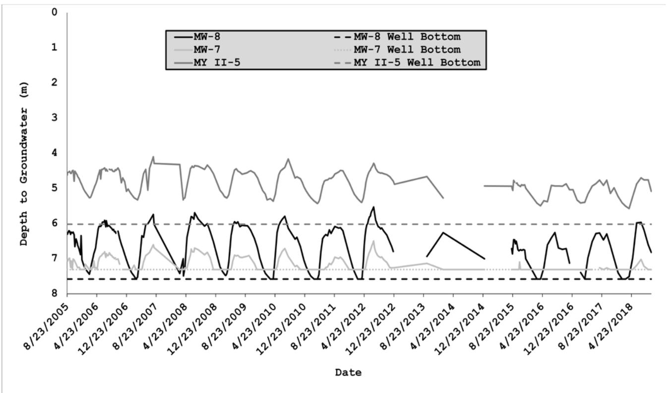
Figure 28. Depth to groundwater at three monitoring locations in the terrace zone at Aztec Ruins NM from August 2005 to October 2018.
