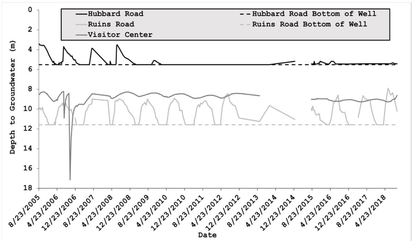
Figure 27. Depth to groundwater at three locations in the terrace zone at Aztec Ruins NM from August 2005 to October 2018.
