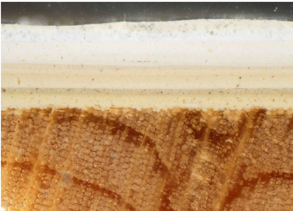
Figure 11. Sample HCS.12, representing typical finish layers for interior first floor surrounds, similar to samples HCS.11 and HCS.15. Note early cream and tan colored finishes and subsequent white finishes. Visible light, 40x magnification.
