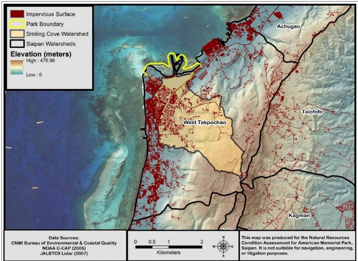
**Figure 31.** Map of the West Takpochao watershed and impervious surfaces. The area of impervious surface is high in the park’s watershed, the West Takpochao watershed. The stormwater drainage system in the park is frequently overwhelmed during heavy rainfall. This is causing extreme stormwater drainage issues, including contamination, sedimentation, and flooding. Graphic is figure 16 from Greene et al. (2019).
