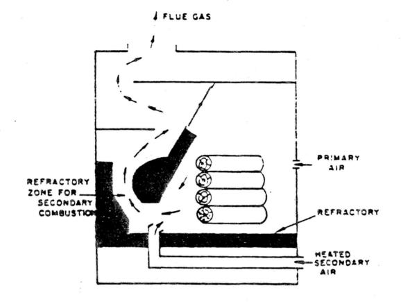
Figure 3. Non-catalyst design wood stove. (A.C.S. Hayden and R. W. Bratten -Reference 2.)
