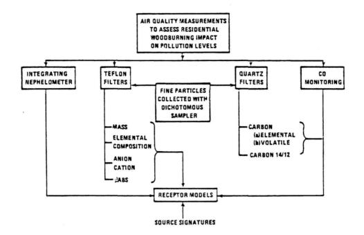
Figure 1. Flow diagram of sampling and analysis needed to support receptor modeling related to residential wood burning. (R. K. Stevens - Reference 10).
