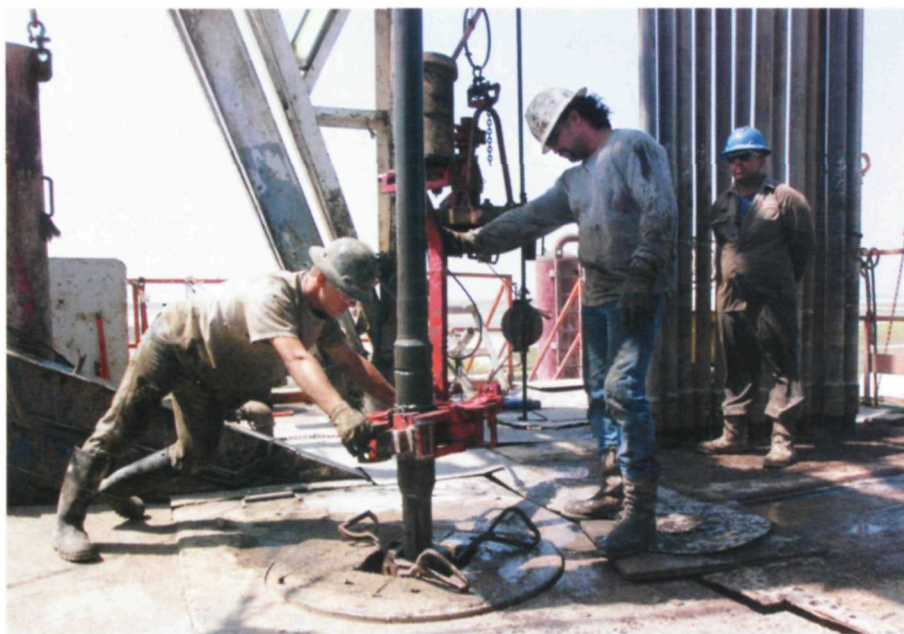
A drill pipe is added to increase the depth of the gas rig on Padre Island National Seashore.
