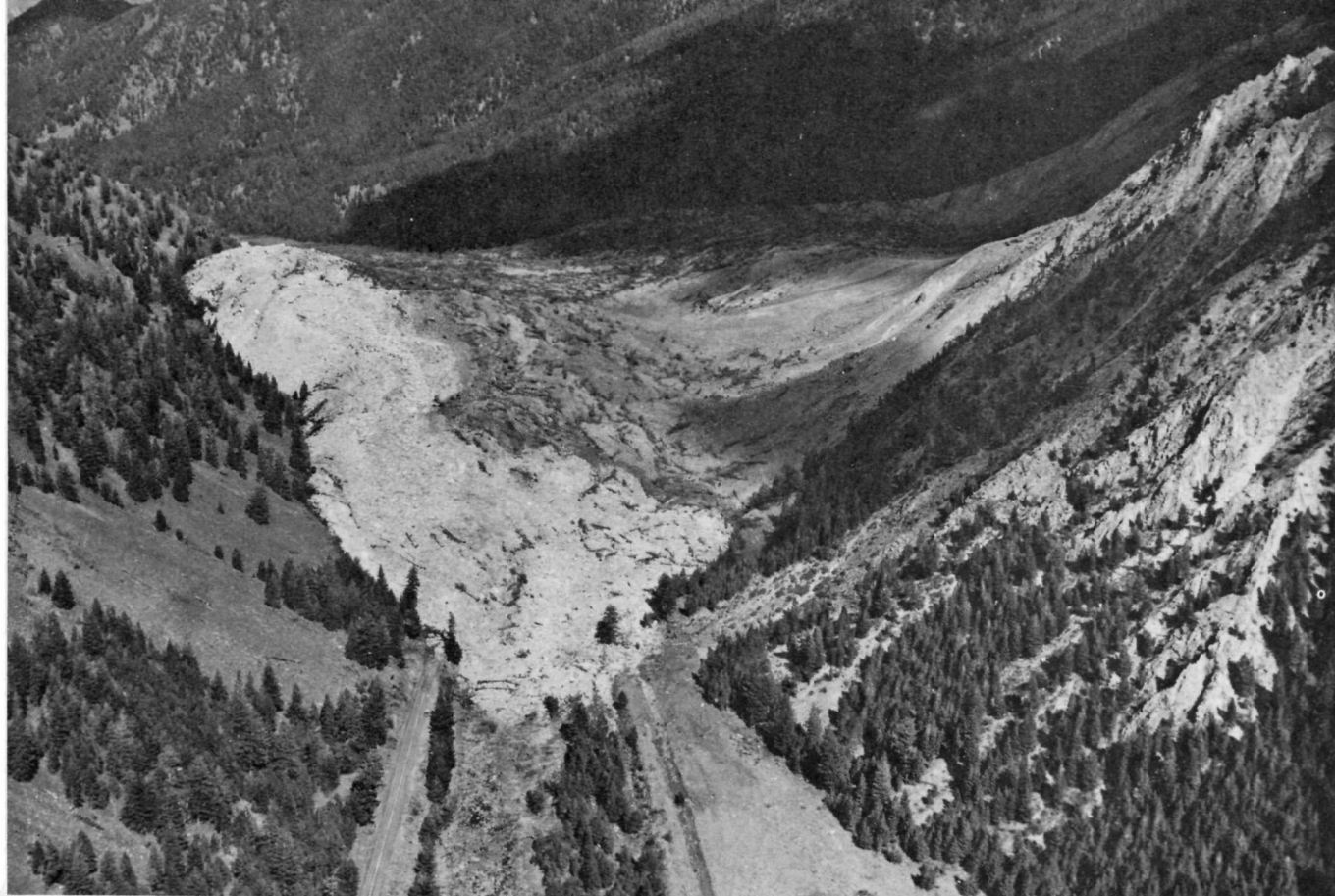
Downstream face and top of landslide. Note pickup truck on highway and the dry bed of the Madison River paralleling highway.
