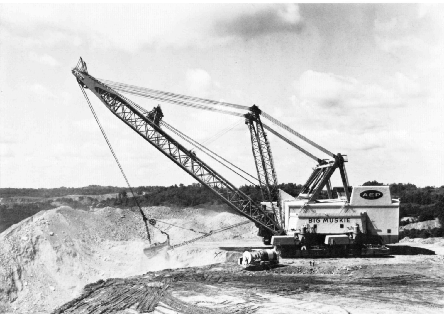
The largest mobile land machine in the world digs for coal near Zanesville, Ohio, while two men watch. "Big Muskie" is 10 stories tall, as wide as an eight-lane highway, and has a bucket that can hold 325 tons of earth and rock. Ohio Power Company built the giant machine to provide coal for an electric power plant.
