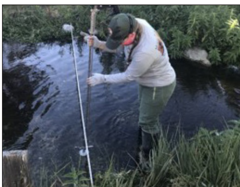
Masked Physical Scientist practicing a new method of taking discharge measurements during an annual streams monitoring visit to Great Basin National Park. Photo: B. Roberts.
