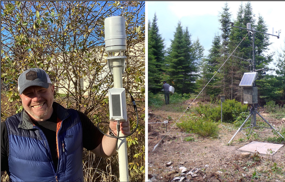
GLKN began pilot testing a new weather monitoring system this spring. While the football-sized unit would still be mounted on a tower to give it clear access for communication, the modern ClimaVue50-Aspen10 from Campbell Scientific ( left ) would consolidate all the sensors into that single unit, would eliminate a control panel box, and has a smaller solar panel than the weather stations placed in parks in the mid-2000s ( right ). NPS PHOTOS
