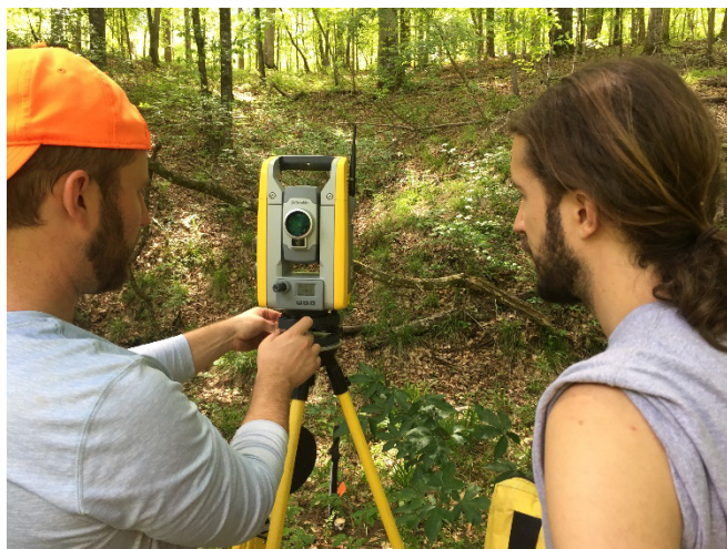
Fluvial geomorphologist Jake McDonald, left, and hydrologic technician Daniel McCay, right, check out a total station during wadeable stream habitat and suitability survey at Horseshoe Bend Military Park on April 23. NPS photo / Eric Starkey
