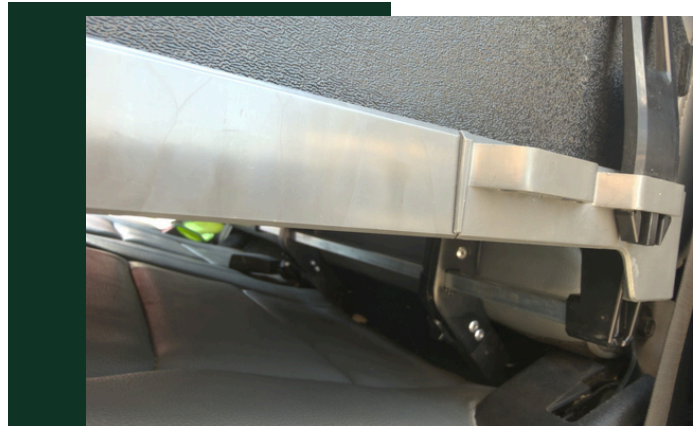
The Karga secured into the child seat anchor system
