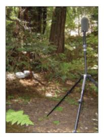
A soundscape monitor set up at Muir Woods National Monument. Note the microphone and tripod in the foreground. The white boxes in the background contain the computer (to capture digital sound data) and batteries to power the system.
