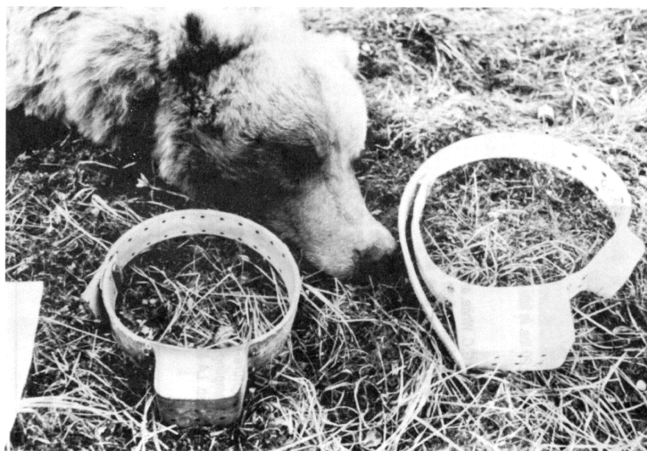
Radio collars and a drugged grizzly bear. A conventional radio collar is on the right. A collar with both conventional and satellite transmitters is on the left.
