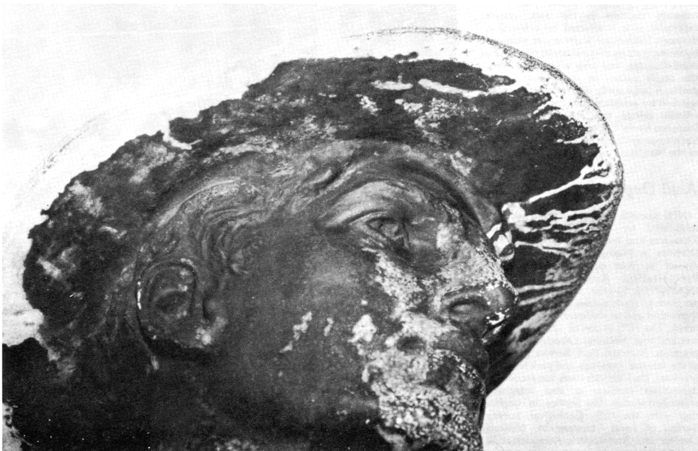
Head of a bronze statue, "The Hiker," honoring soldiers of the Spanish-American War. One of 50 such statues in the U.S., this one, erected in Allentown, PA, in 1937, has suffered pitting on the face and streaking on the hat due to air pollution.
