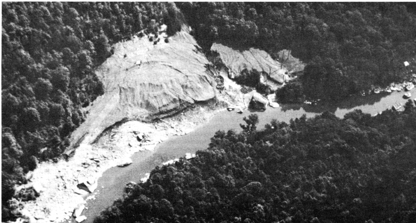
Mine spoil embankments along the Big South Fork of the Cumberland River, Big South Fork NRRA. The highly acidic, pyritic shale in these spoils prevents natural revegetation and adds to erosion and acid runoff problems.
