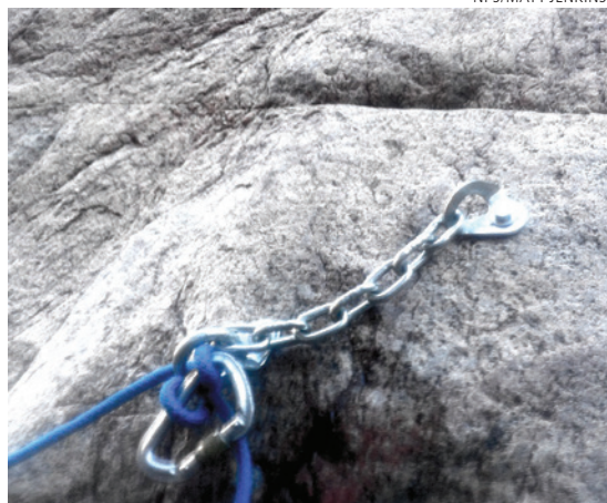
Figure 4. A bolted rappel anchor consisting of two bolts, two hangers, a rappel ring, and a chain are shown with a canyoneering rope and carabiner in Garden Creek in 2013. This Specific fixed anchor configuration was placed at numerous locations in 2013.
