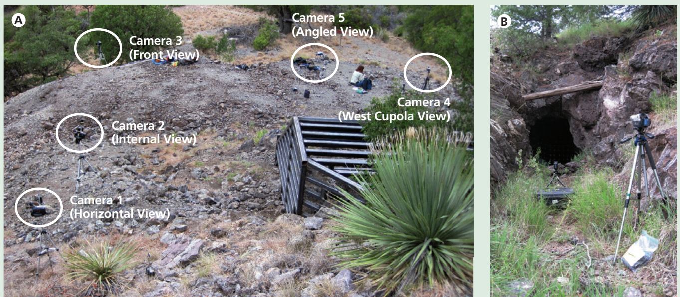
Figure 5. (A) This image shows the locations of cameras 1 through 5. (B) The photo at the right shows the location of video camera 6 at the lower adit. Note: In 2010, camera 3 was positioned to capture the entire gate structure and surrounding area; It was later repositioned closer to the front gate to obtain a better view of the front of the gate.
