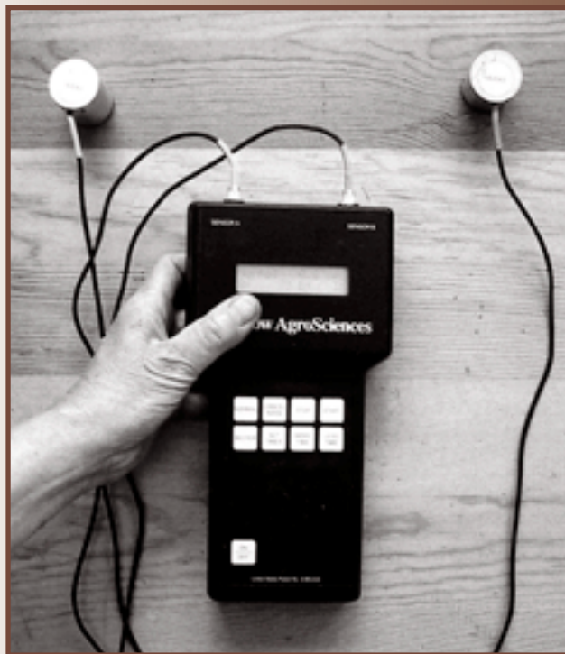
Figure 6. The acoustic emission detector (AED) recorded sound waves that were generated when wooden fibers were broken by termite mandibles, and was used to measure termite feeding in wood.
