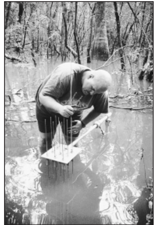
Figure 1. A wetlands ecologist from the National Wetlands Research Center measures soil elevations for baseline assessments at Big Thicket National Preserve, Texas. Known as a sedimentation-erosion table, the device depicted is used in conjunction with marker horizon techniques to measure accretion, erosion, and subsidence at wetland sites. Data are being collected to determine the sediment budget for the Neches River floodplain as part of a larger study of water quality.
