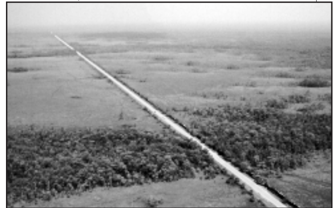
Figure 3. Built in the 1920s, the two-lane Tamiami Trail interrupts the natural north-south flow of water through Big Cypress National Preserve and Everglades National Park. Improving the conveyance of sheetflow through the highway is a critical aspect of ecological restoration in the preserve.
