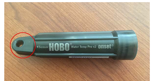
Onset U22 data logger with the sensor end circled in red.
